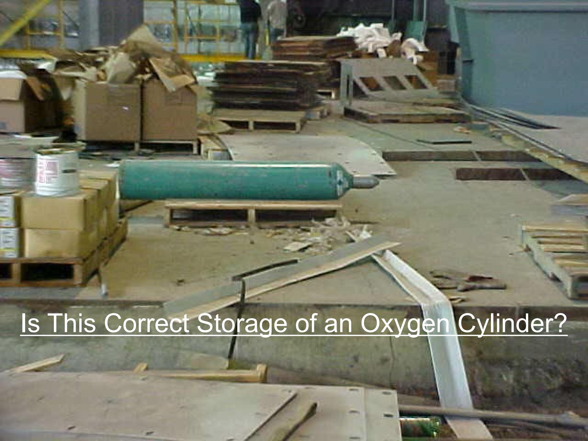
Is This Correct Storage of an Oxygen Cylinder?
