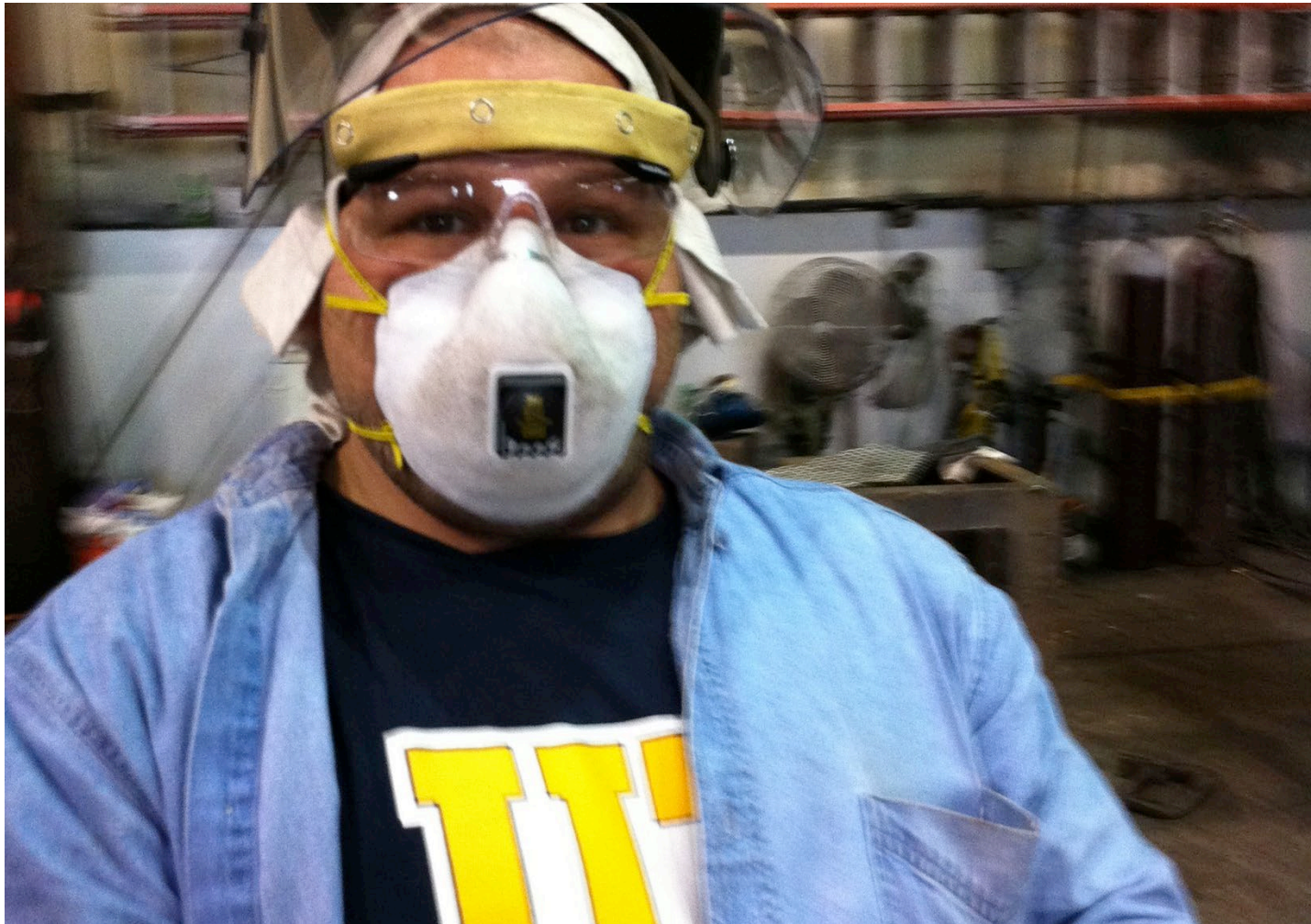
Welder Wearing Respirator During Welding of Stainless Steel – Exposure is 56 ug/m 3 of Hex
