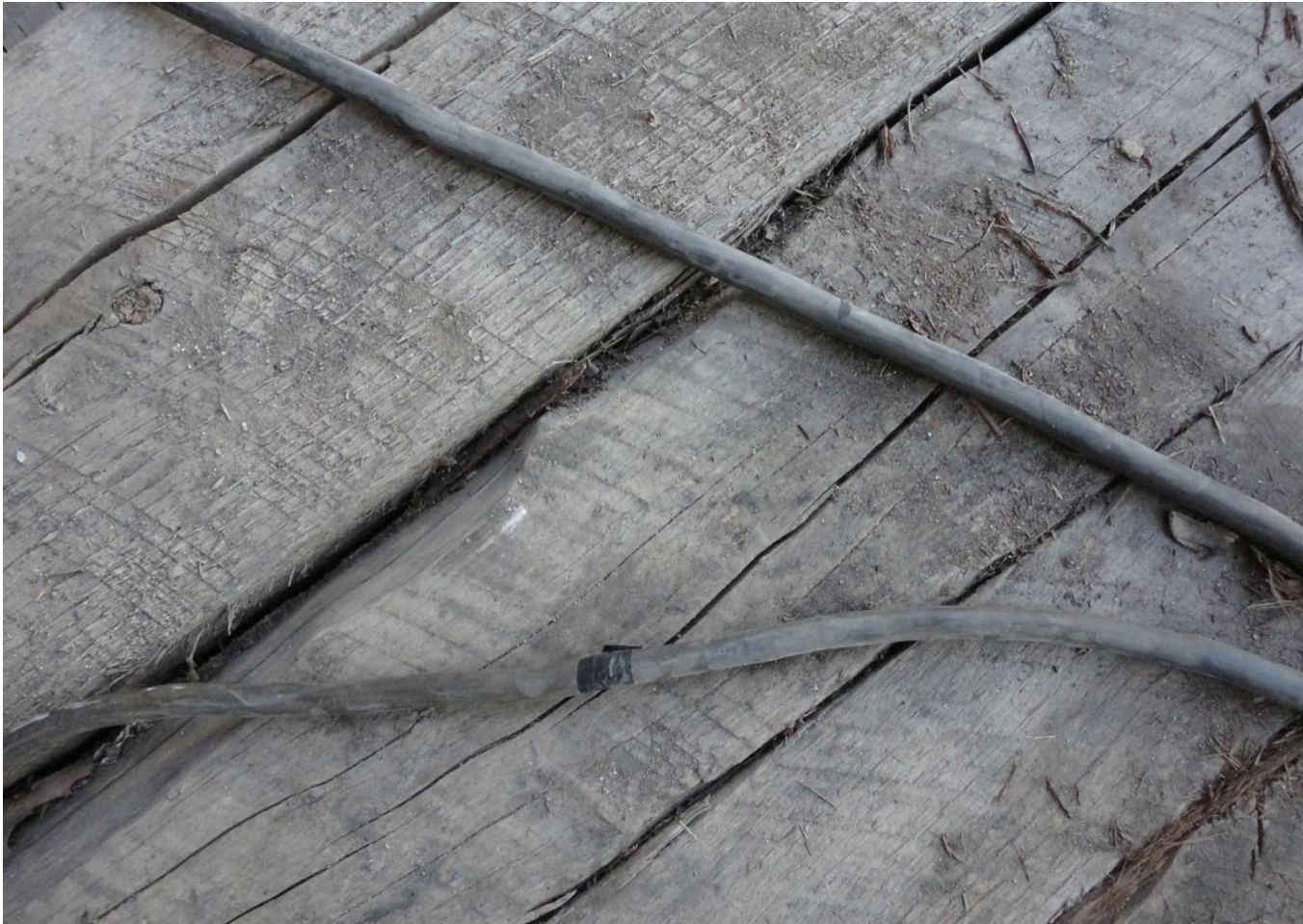
Welding Lead Repaired within 10 ft. of the Stinger
