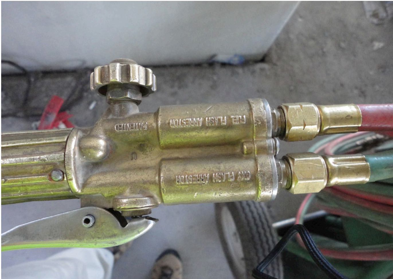
Flash Arrestors in Torch Head – None at Gauges
