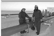
Photo Courtesy of Yxlon International Radiography of weld joints.
