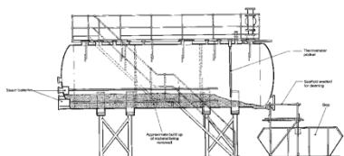
Figure 8 Longitudinal section of 60,000-barrel oil base showing estimated sludge accumulation and position of the thermometer jacket
