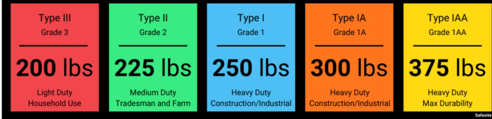
*A guide to ladder duty rating labels. See the label on your ladder to determine its maximum load.*
