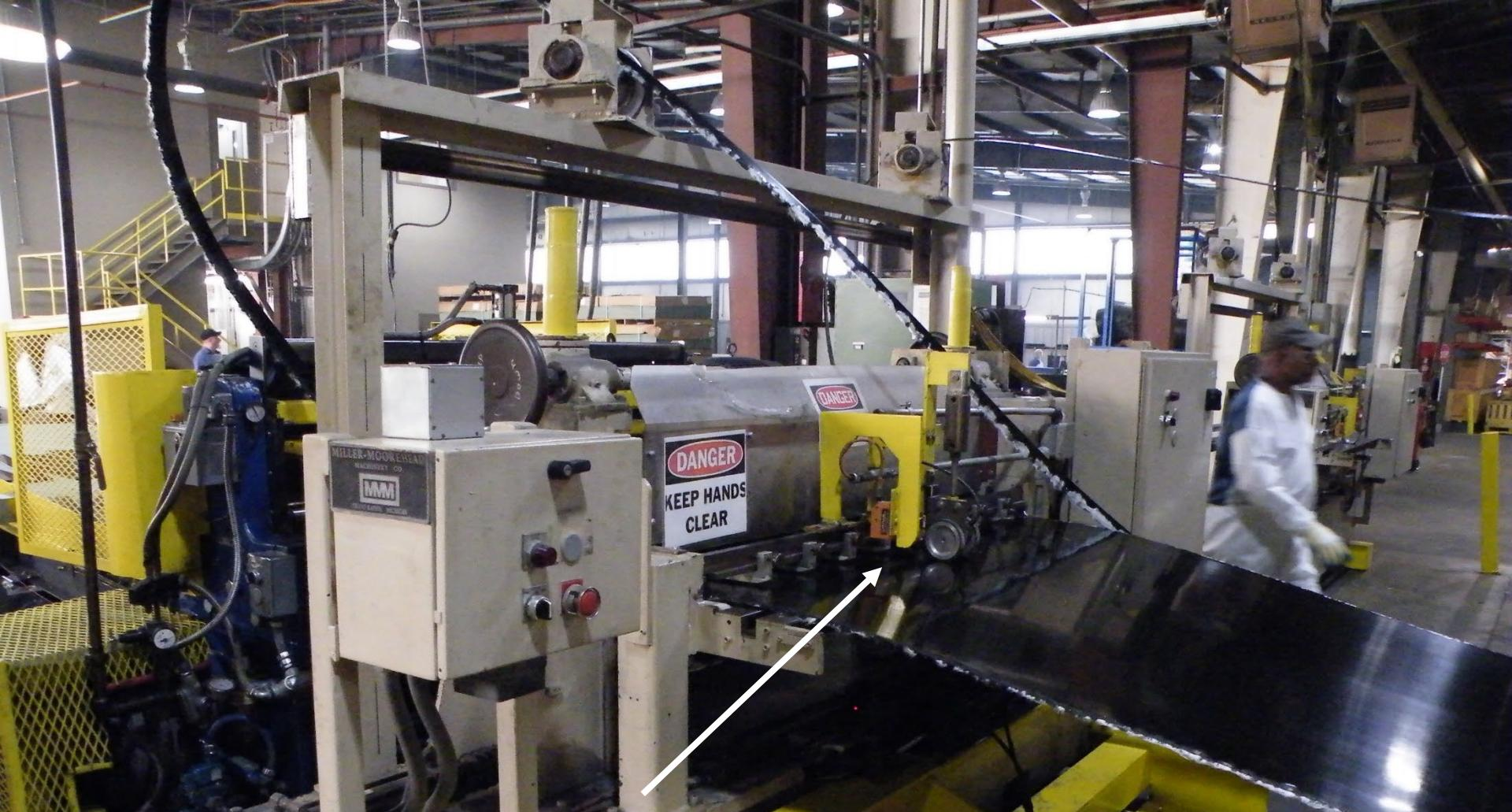
Thermoplastic material coming into the slitter is cut it into specified widths. It then goes to the vertical shear. A “bow-up” occurs at this location when there is a break in the material in the slitter or a mis-feed from the slitter to the shear.
