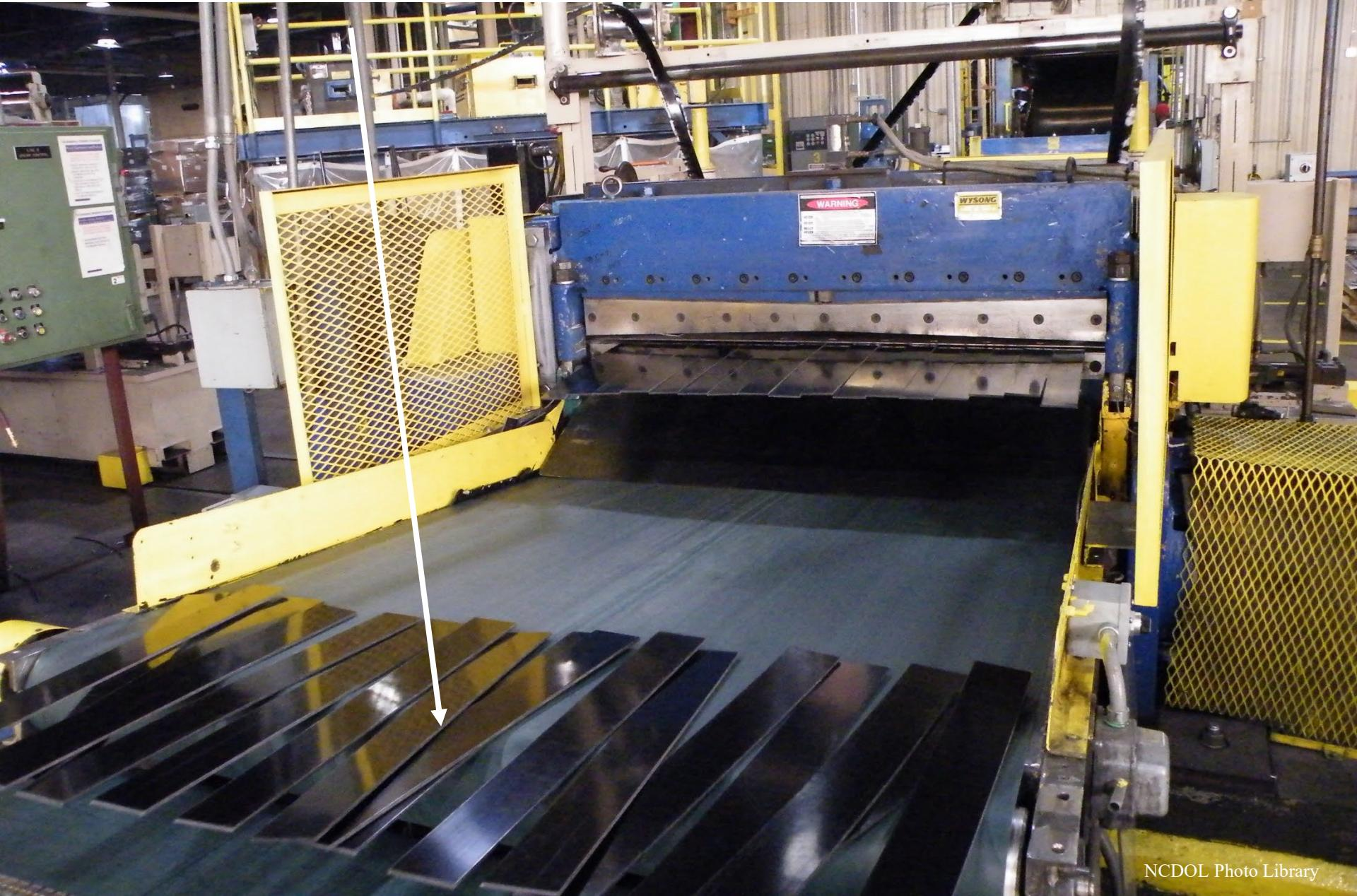
Thermoplastic material after going through the slitter and shear.
